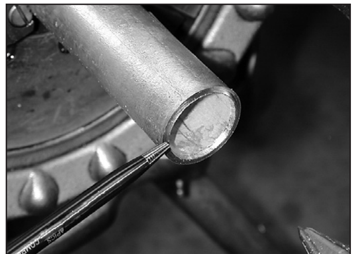
Figure 8: A minimal amount of pressure will remove the burr completely and eliminate possible flaring of the conduit end.
