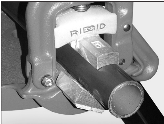
Figure 14: Commercial yoke vise used to protect the PVC coating of PVC-coated conduit.
