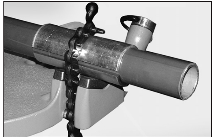
Figure 15: Field-fabricated half shell clamps used with chain vise to protect PVC-Coated conduit.
