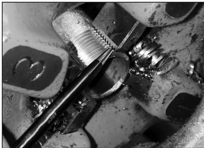
Figure 9: When proper thread length is achieved the end of the conduit becomes flush with the ends of the die segments.
