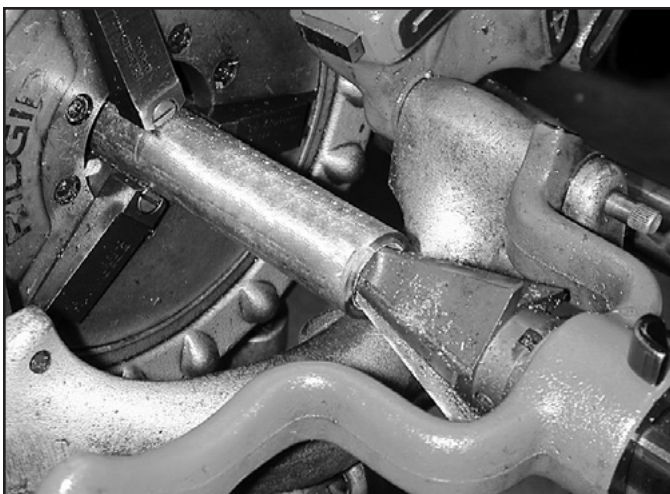
Figure 7: Insert the (flute) reamer into work piece and rotate until burr is removed.
