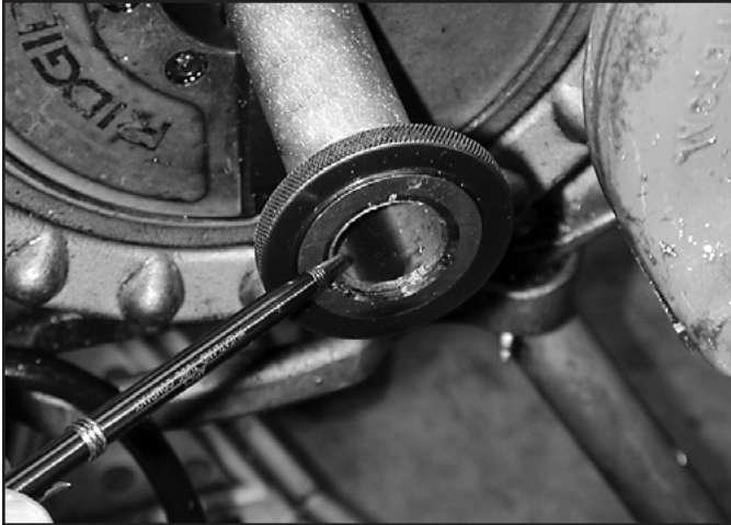
Figure 11: Threads should be checked with a NPT-L1 threaded ring gauge to ensure proper make up.
