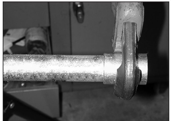
Figure 13: The coupling must be assembled wrench tight.
